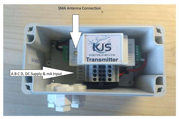
Step 1: Mount the Tx close to the instrument measuring the process, supplying a 4 to 20mA signal.
