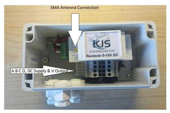
Step 1: Mount the Rx close to the monitoring station that requires the 0-10V output.
