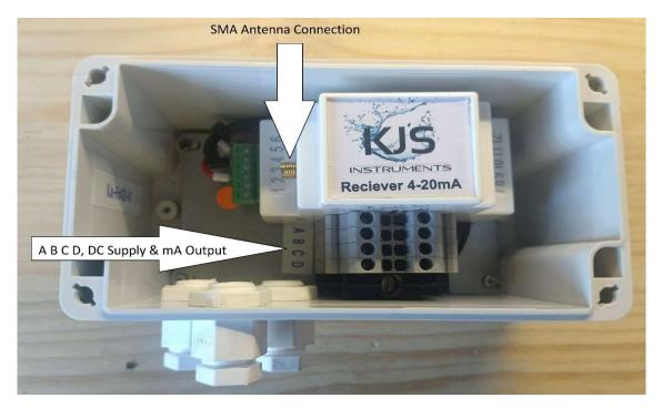
Step 1: Mount the Rx close to the monitoring station that requires the 4 to 20mA output.
